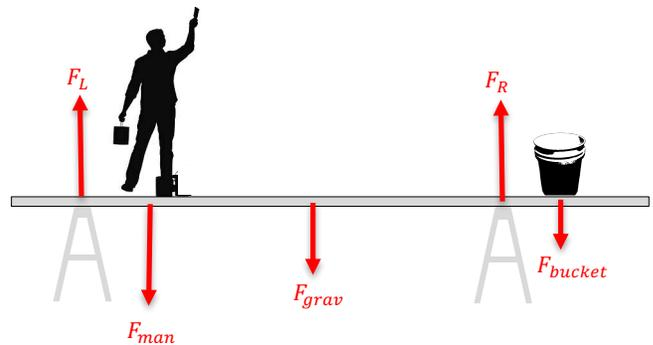
a) The sawhorses are holding up 100 kg, which exerts a force of 1000 Newtons. To get the force the left sawhorse exerts on the plank, the most straightforward method is to take torques about the sawhorse on the right.
